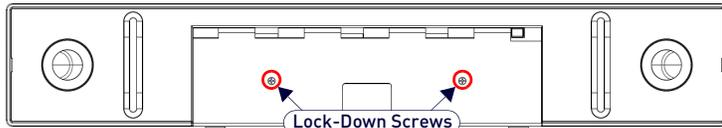
FIG. 7 ACV-2100 BOTTOM VIEW - LOCK DOWN SCREW LOCATIONS
