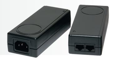
When you need to get power and data through a single cable to remotely located Power-over-Ethernet (PoE)enabled devices, look no further than the AMX PoE Injector. This single port, self-contained PoE gigabit power supply "injects" DC power and data through the same Cat 5 Ethernet cable, eliminating the need for an AC outlet at each end device location. This results in easier installation, less wiring and a decrease in installation cost.
