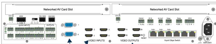
Six video inputs: two VGA and four HDMI
