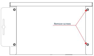
4. Align and secure the second mounting wing to the bottom of unit, using the same two screws you just removed. Make sure the screws are tightened properly.
