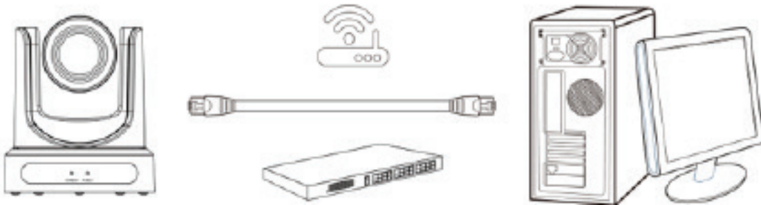
Picture 1.2 Connections to LAN via patch cable to LAN wall jack or LAN Switch
