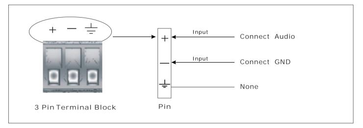
Receiver (Audio): 1-Channel Simplex Audio Connection (Output)
