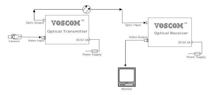
The VOS-1000FT transmitter/VOS-1000FR receiver can be mounted into a rack or can be used as a stand-alone module. As a stand-alone module, the unit can be placed on a desktop or can be mounted to a wall.
