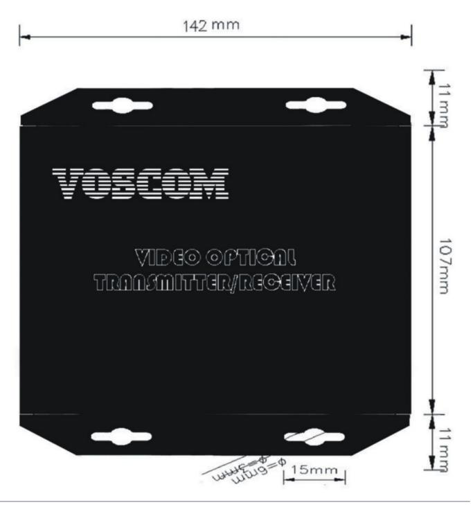
The VOS-10101FDET transmitter/VOS-10101FDER receiver can be installed into our rack mount chassis, VOS-CH04 or VOS-CH06, which can be mounted into an industry-standard 19-inch equipment rack.
