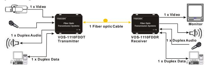
NOTE1: Digital video optic transmitter and receiver should be used in pairs, one is Transmitter (LED is red), the other is Receiver (LED is green).
