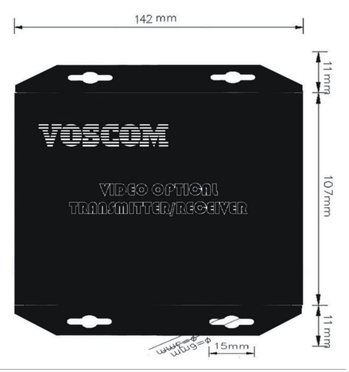
The VOS-1110FDDT transmitter/VOS-1110FDDR receiver can be installed into our rack mount chassis, VOS-CH04 or VOS-CH06, which can be mounted into an industry-standard 19-inch equipment rack.
