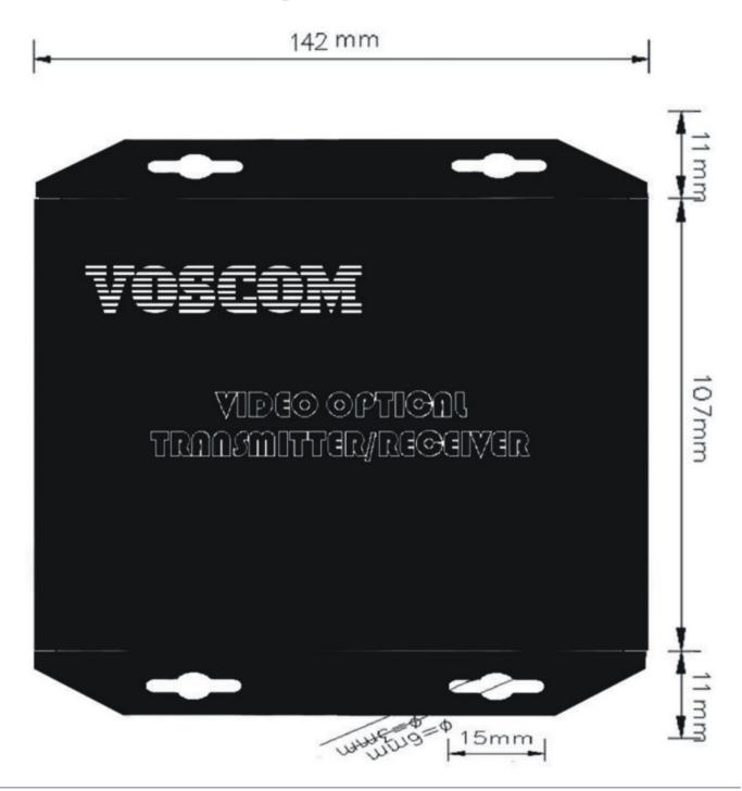
The VOS-1110FFDT transmitter/VOS-1110FFDR receiver can be installed into our rack mount chassis, VOS-CH04 or VOS-CH06, which can be mounted into an industry-standard 19-inch equipment rack.
