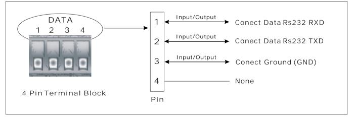
Receiver (Rs232): One Duplex Rs232 Data Connection (Input/Output)
