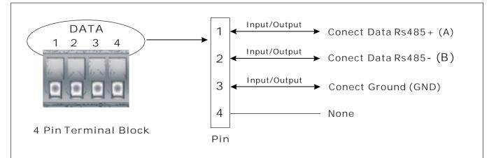
Receiver (Rs485): One Duplex Rs485 Data Connection (Input/Output)
