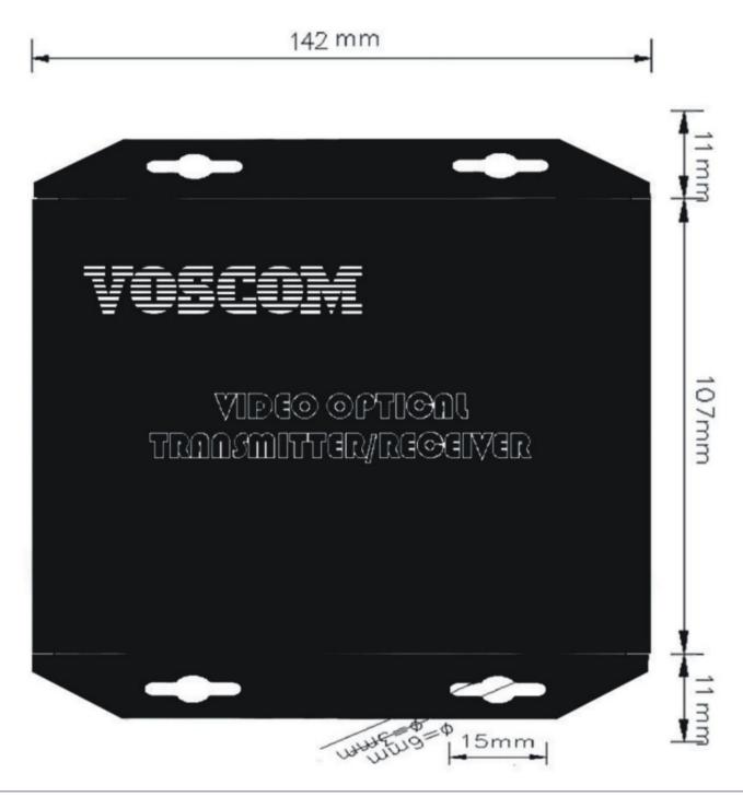
The VOS-22101FDDET transmitter/VOS-22101FDDER receiver can be installed into our rack mount chassis, VOS-CH04 or VOS-CH06, which can be mounted into an industry-standard 19 inch equipment rack.
