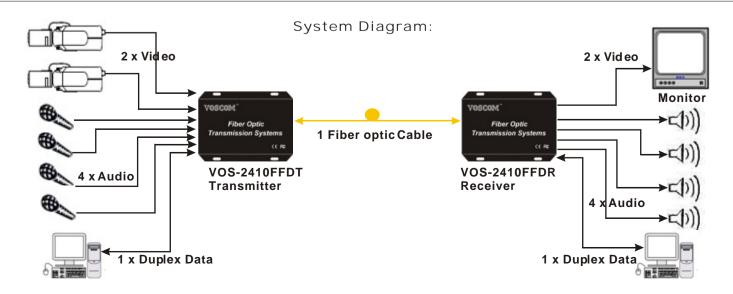
NOTE1: Digital video optic transmitter and receiver should be used in pairs, one is Transmitter (LED is red), the other is Receiver (LED is green).
