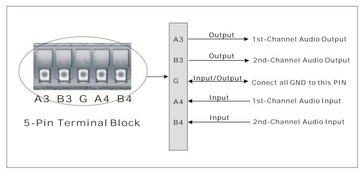
Receiver (Audio): 2-Channel Duplex Audio (Input/Output)
