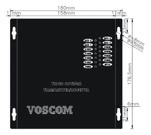
The VOS-40101FDET transmitter/VOS-40101FDER receiver can be installed into our rack mount chassis, VOS-CH04 or VOS-CH06, which can be mounted into an industry-standard 19-inch equipment rack.
