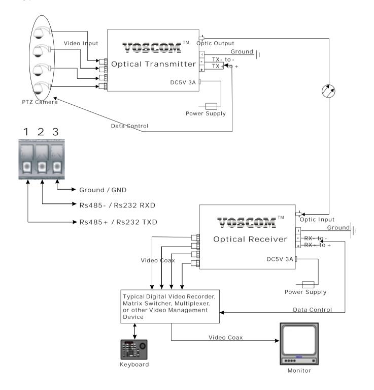
The VOS-4010FDT transmitter/VOS-4010FDR receiver can be mounted into a rack or can be used as a stand-alone module. As a stand-alone module, the unit can be placed on a desktop or can be mounted to a wall.
