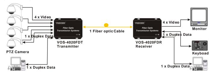
NOTE1: Digital video optic transmitter and receiver should be used in pairs, one is Transmitter (LED is red), the other is Receiver (LED is green).
