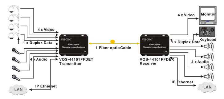
NOTE1: Digital video optic transmitter and receiver should be used in pairs, one is Transmitter (LED is red), the other is Receiver (LED is green).
