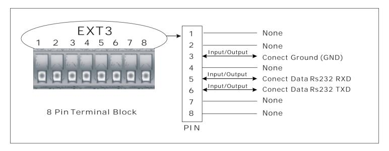
Receiver (Rs232): One duplex Rs232 Data Connection (Input/Output)
