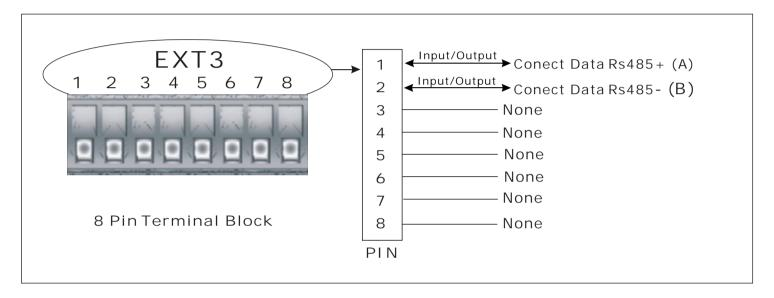
Receiver (Rs485): One duplex Rs485 Data Connection (Input/Output)
