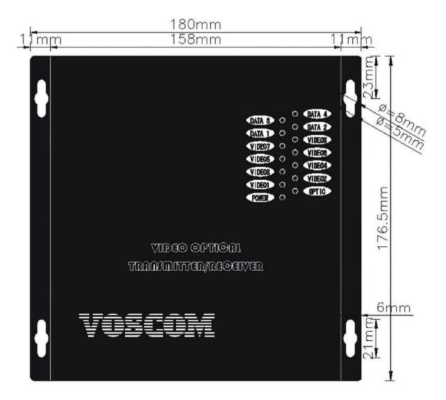
The VOS-8010FDT transmitter/VOS-8010FDR receiver can be installed into our rack mount chassis, VOS-CH04 or VOS-CH06, which can be mounted into an industry-standard 19-inch equipment rack.
