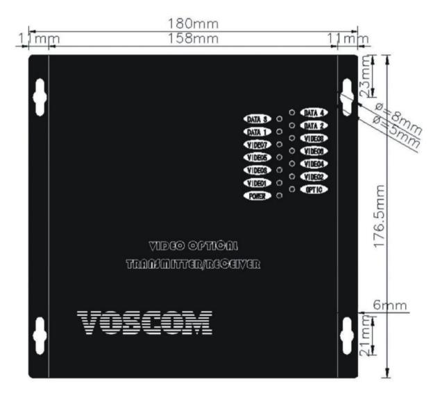
The VOS-88101FFDET transmitter/VOS-88101FFDER receiver can be installed into our rack mount chassis, VOS-CH04 or VOS-CH06, which can be mounted into an industry-standard 19-inch equipment rack.
