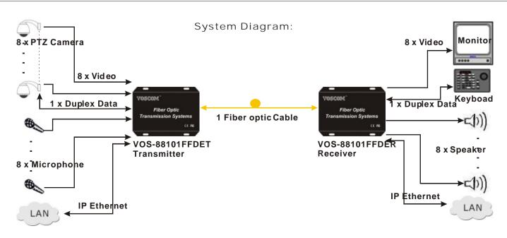
NOTE1: Digital video optic transmitter and receiver should be used in pairs, one is Transmitter (LED is red), the other is Receiver (LED is green).
