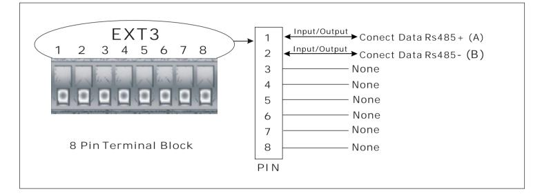
Receiver (Rs485): One duplex Rs485 Data Connection (Input/Output)
